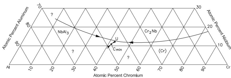
**Fig. 1** Al-Cr-Nb partial liquidus projection for Nb-lean alloys [2006Sou]
