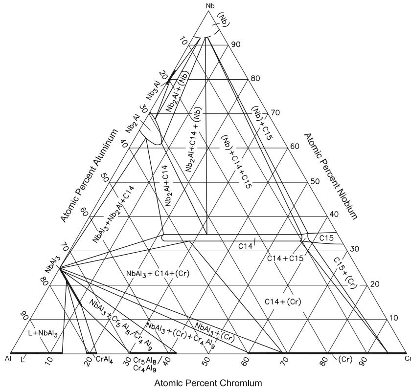
**Fig. 2** Al-Cr-Nb isothermal section at 1000 °C [2001Mah, 2004Zha]
